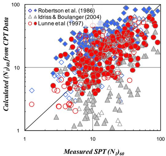
Figure 3. Comparison of measured and calculated  $(N_1)_{60}$
