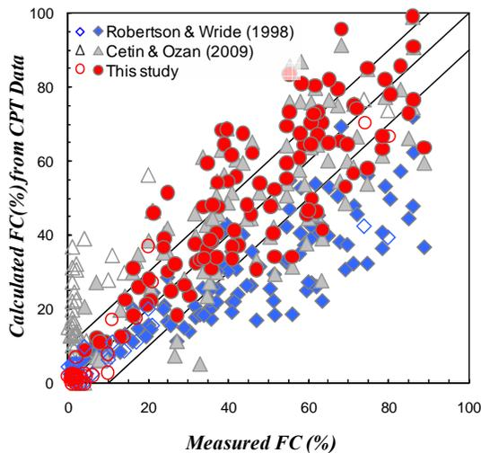
Figure 2. Comparison of measured and calculated fines content
